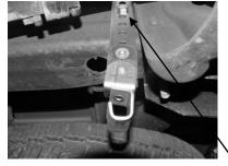
INSTALL METAL HANGERS #H INTO HOLES LOCATED APPROX. 16" FROM THE REAR OF THE FRAME. METAL HANGERS ARE MOUNTED ON THE OUTSIDE OF FRAME. USE THE HARDWARE PROVIDED. THE BOLT AND WASHER WILL GO INTO THE 3<sup>RD</sup> HOLE FROM THE TOP OF THE HANGER. YOU MAY NEED TO LOOSEN SPARE TIRE FOR EASIER REMOVAL.
