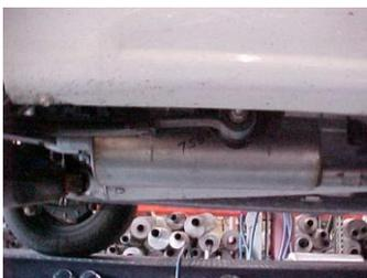
Install muffler onto head pipe 1-1/2" to 2" with the louvers facing towards the converter. Use a jack stand to support the muffler. Use clamp (#G) to secure the muffler to the head pipe. Do not tighten
