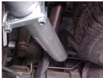
Install the driver side tailpipe (#D) into the muffler at least 1-1/2" to 2". This pipe will route over the axle and between the shock and tire. Use clamp # F to secure pipe to the muffler. Do not tighten.
