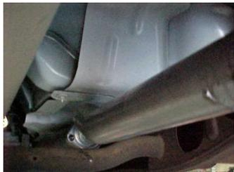
Install head pipe (#A) onto your existing stock flange use your factory hardware. Use a jack stand to support the converter. Insert welded hanger into rubber grommet. Do not
