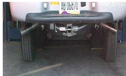
Install exit pipes (#E) Use clamps (#H) to secure exit pipes to tailpipes. These clamps also attach to the metal hangers' (#I). You will need to rotate in order to adjust for clamping. Now go back and tighten all clamps, nuts and bolts. Start from the front and work back. Install Stainless tips.
