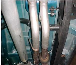
Install driverside headpipe #B. Then install headpipe #A and insert welded hanger into rubber grommet. Secure both pipes with clamp #H. Do not tighten.
