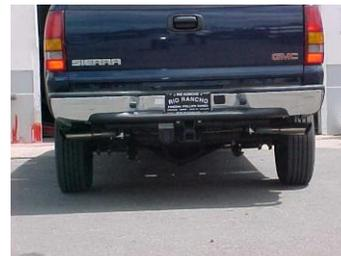
Install exit pipes #F. Use clamps #I to attach to tailpipes. These clamps also attach to the metal hangers # J. Rotate to adjust for clamping. Now go back and tighten up all clamps, nuts, and bolts.
