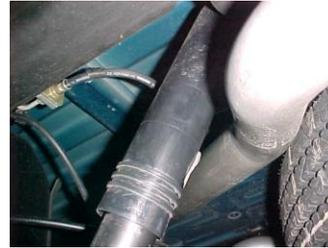
Install driverside overaxle tailpipe #E into muffler 1 1/2" to 2". Use clamp #I to secure pipe to muffler. Do not tighten. Next, insert welded hanger into rubber grommet. Rotate pipe until it connects to rear hanger #J. Attach clamp #I to pipe.
