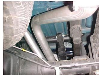
Install passenger side overaxle tailpipe #D into muffler 1 1/2" to 2". Secure to muffler with clamp #I. Do not tighten. Next rotate pipe until it connects to rear hanger #J. Use clamp #J to hold up pipe.
