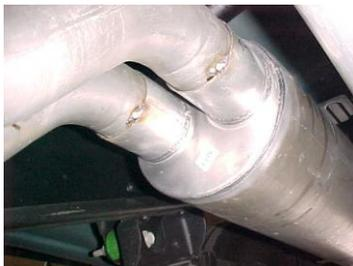
Install muffler# C onto head pipes 1-1/2" to 2" with the louvers facing towards the converter. Use a jack stand to support the muffler. Use clamps #G to secure the muffler to the head pipes. Do not tighten
