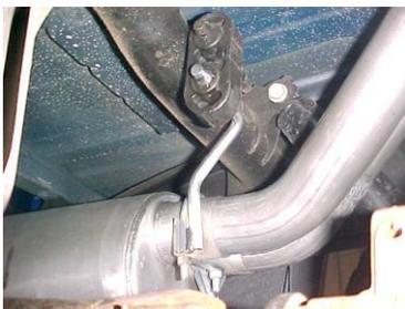
SLIDE MUFFLER #C ONTO HEADPIPES 1-1/2" TO 2", WITH THE INLET FACING THE MOTOR, USE A JACK STAND TO SUPPORT MUFFLER. USE CLAMP #G TO SECURE MUFFLER TO HEADPIPES. DO NOT TIGHTEN. OUTLETS OF THE MUFFLER SHOULD BE ON THE TOP. THE INLET OF THE MUFFLER IS LOOKING INTO THE LOUVERS. INSTALL REAR MUFFLER HANGER # J ONTO DRIVERSIDE OUTLET. DO NOT TIGHTEN.
