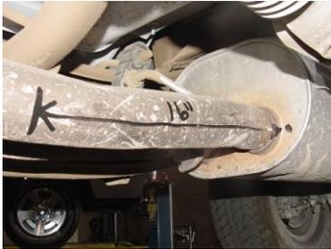
**TO REMOVE STOCK EXHAUST, CUT 16" FROM THE FRONT OF THE MUFFLER FORWARD TOWARDS THE FRONT OF THE VEHICLE. LEAVE ALL RUBBER GROMMETS ON THE HANGERS. USE WD-40 TO AID IN THE REMOVAL OF EXHAUST AND HANGERS.**
