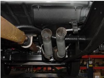
SLIDE PASSENGER SIDE HEADPIPE #A ONTO STOCK HEADPIPE. INSERT WELDED HANGER INTO RUBBER GROMMET. NEXT INSTALL DRIVERS SIDE HEADPIPE #B ONTO STOCK HEADPIPE. USE CLAMP #I TO SECURE BOTH HEADPIPES, DO NOT TIGHTEN.
