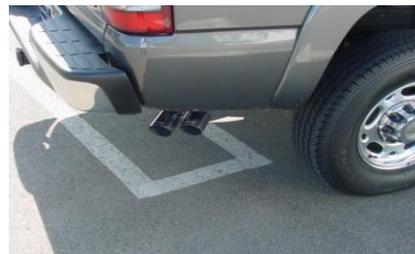
INSTALL YOUR STAINLESS STEEL TIPS. TO CLEAN TIPS USE A SCOTCH BRITE PAD AND ANY STAINLESS OR ALUMINUM CLEANER. AFTER YOU HAVE CHECKED FOR CLEARANCES GO BACK AND TIGHTEN ALL NUTS, BOLTS. TIGHTEN CLAMPS TO APPX 100-150 FT LBS .
