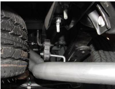
SLIDE PASSENGER SIDE TAILPIPE #E INTO OUTLET OF MUFFLER 1-1/2" TO 2". INSERT WELDED HANGER INTO RUBBER GROMMET. USE CLAMP #G TO SECURE TAILPIPE TO MUFFLER. DO NOT TIGHTEN.
