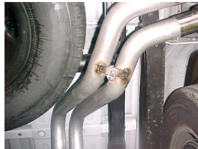
BOLT THESE TOGETHER USING BOLT KIT #H.
