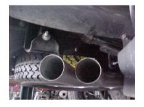
SLIDE DRIVERS SIDE TAILPIPE #B INTO MUFFLER 1-1/2" TO 2". NEXT SECURE TAILPIPE TOGETHER WITH BOLT KITS # H THE DRIVERS SIDE TABS ON PIPE SHOULD BE ON THE **BOTTOM PASSENGER** SIDE TAB.ON THE TOP. SECURE DRIVERS SIDE PIPE TO MUFFLER WITH REAR MUFFLER HANGER # E. DO NOT TIGHTEN.
