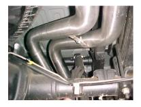
SLIDE PASSENGER SIDE TAILPIPE #C INTO MUFFLER 1-1/2" TO 2" AND INSERT WELDED HANGER INTO RUBBER GROMMET. USE CLAMP #F TO SECURE TAILPIPE TO MUFFLER. DO NOT TIGHTEN.
