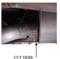
TO REMOVE STOCK EXHAUST, CUT OFF YOUR STOCK SYSTEM JUST IN FRONT OF THE MUFFLER AFTER THE WELD. LEAVE ALL RUBBER GROMMETS ON THE HANGER. USE WD-40 TO AID IN THE REMOVAL OF EXHAUST AND HANGERS.
