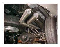
SLIDE DRIVERS SIDE TAILPIPE #C INTO MUFFLER 1-1/2" TO 2". SECURE WITH CLAMP #G. USE BOLT KIT #H TO SECURE THE TAILPIPES TOGETHER. THE TABS ON THE DRIVERS SIDE TAILPIPE SHOULD BE ON THE BOTTTOM.
