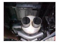
INSTALL MUFFLER #A ONTO STOCK HEADPIPE. USE CLAMP #E TO SECURE MUFFLER TO THE HEADPIPE. DO NOT TIGHTEN.
