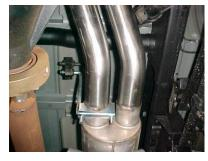
SLIDE PASSENGER SIDE TAILPIPE #B INTO MUFFLER 1-1/2" TO 2". USE CLAMP #F TO SECURE TAILPIPE TO MUFFLER. DO NOT TIGHTEN.
