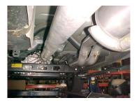
Install passenger side head pipe # A onto you're existing stock flange use bolt kit # J to secure it. Do not tighten. Use a jack stand to support the converter. Insert welded hanger into rubber grommet. Next, install driver side # B onto stock pipe. Use clamp # G to secure. Do not tighten.
