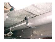
INSTALL DOWNPIPE #B ONTO PIPE #A. USING GASKET #J AND BOLT KIT #I INSERT WELDED HANGERS INTO RUBBER GROMMETS.
