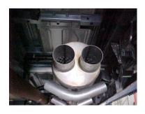
INSTALL MUFFLER #C ONTO PIPE #M. USE CLAMP #K TO SECURE MUFFLER TO THE HEADPIPE. DO NOT TIGHTEN.
