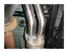
SLIDE PASSENGER SIDE TAILPIPE #E INTO MUFFLER 1-1/2" TO 2". USE CLAMP #G TO SECURE TAILPIPE TO MUFFLER. DO NOT TIGHTEN.
