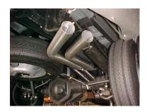
SLIDE DRIVERS SIDE TAILPIPE #D INTO MUFFLER 1-1/2" TO 2". SECURE WITH CLAMP #L. USE BOLT KIT #H TO SECURE THE TAILPIPES TOGETHER. THE TABS ON THE DRIVERS SIDE TAILPIPE SHOULD BE ON THE BOTTTOM.
