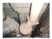
TO INSTALL YOUR GIBSON DOWN PIPE YOU NEED TO REMOVE YOUR STOCK EXHAUST. REMOVE IT FROM THE 4 BOLT FLANGE IN FRONT OF YOUR STOCK MUFFLER. CUT OFF YOUR STOCK TAILPIPE FOR EASIER REMOVAL. LEAVE ALL RUBBER GROMMETS IN PLACE. USE WD-40 TO AID IN REMOVAL OF EXHAUST AND HANGER.
