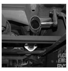
BOLT HEADPIPE #A TO STOCK FLANGE USING GASKET # F AND RE-USING STOCK NUTS AND BOLTS. INSERT WELDED HANGER INTO RUBBER GROMMETS.
