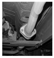
TO REMOVE **EXHAUST-UNBOLT THE** FLANGE LOCATED **BEHIND THE CATALITIC** CONVERTER. **SAVE STOCK NUTS AND BOLTS FOR YOU WILL** REUSE THEM. NOW CUT OFF YOUR STOCK TAILPIPE JUST **BEHIND THE** MUFFLER AND REMOVE. LEAVE ALL RUBBER **GROMMETS ON** THE HANGER. USE WD-40 TO AID IN THE REMOVAL OF THE **EXHAUST AND** HANGERS.
