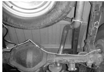
Slip the over axle tailpipes #C, #D into the outlets of the muffler no more than 1- 1/2" to 2" and attach clamp # G to passenger side and clamp hanger # I to driver side tailpipe.
