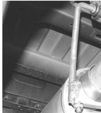
Install hanger #I onto the rear outlet of the muffler on the driver side. Insert the vertical rod through the rubber grommet from the driver side towards the passenger side. Do not tighten.
