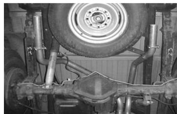
Install exit pipes # E onto the over axle pipes and attach with clamp #G. You may need to cut the exit pipes to your preference. Rotate all pipes until you have a minimum of a 1" clearance on all pipes. Use zip ties to reroute vent lines and brake lines. Tighten all clamps, flanges, bolts firmly. Stainless steel tips are optional.
