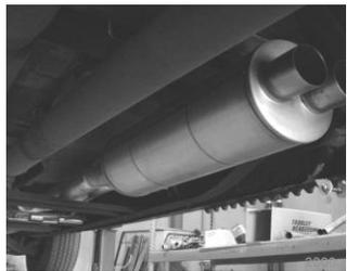
Install the muffler onto the head pipe no more than 1 1/2" to 2". Use a jack stand to support the muffler. Make sure muffler is sitting level with the vehicle and that the muffler outlets are positioned level. Level outlets across at 12'oclock position.
