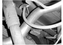
REMOVE THE REAR FACTORY HANGER. INSTALL HANGER #I TO THE BOTTOM STOCK HANGER HOLE. BOLT IT THROUGH THE 5<sup>TH</sup> HOLE DOWN FROM THE TOP OF THE HANGER. REPEAT ON THE DRIVER SIDE.
