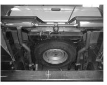
Now install exit pipes #F to tailpipe using clamp #G.
