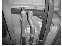
Slide head pipes #A and B over stock headpipes 1-1/2" to 2". Insert welded hanger on driver side headpipe into rubber grommet. Attach headpipe to stock headpipe with clamps #J.
