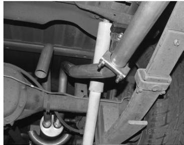
INSTALL PASSENGER SIDE TAILPIPE # C INTO THE MUFFLER 1-1/2" TO 2". ATTACH IT TO THE MUFFLER USING CLAMP # I. USE CLAMP # I TO HOLD TAILPIPE TO HANGER # F. DO NOT TIGHTEN
