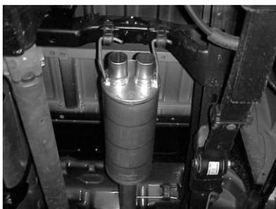
INSTALL MUFFLER # B ONTO HEADPIPE 1-1/2" TO 2" USING CLAMP # J. INSERT WELDED HANGERS INTO RUBBER GROMMET. MAKE SURE OUTLETS ARE LEVEL. USE A JACKSTAND TO SUPPORT MUFFLER. DO NOT TIGHTEN .
