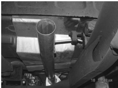
INSTALL HEADPIPE # A USING BOLT KIT # N AND # K GASKET. AND ATTACH TO STOCK FLANGE. DO NOT TIGHTEN.
