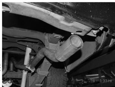
INSTALL EXIT PIPES # H ONTO OVERAXLE TAILPIPES USING CLAMP # I. ADJUST FOR YOUR PREFERENCE. NEXT ROTATE PIPES FOR BEST CLEARANCE AND ALIGN TO FRAME RAIL. TIGHTEN ALL CLAMPS AND BOLTS STARTING FROM THE HEADPIPE AND WORK BACK. INSTALL STAINLESS STEEL TIPS.
