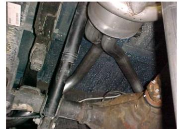
INSTALL DRIVER SIDE OVER AXLE TAILPIPE #D INTO THE MUFFLER. 1 1/2" TO 2" ROTATE PIPE UNTIL IT HITS THE 10" HANGER USE CLAMP # K TO HOLD UP THE PIPE. ATTACH TAILPIPE TO MUFFLER USING CLAMP # J. DO NOT TIGHTEN
