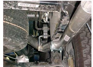
NEXT, INSTALL EXIT PIPES #F ONTO TAILPIPES USE CLAMP # J TO SECURE EXIT PIPES TO TAILPIPES.
