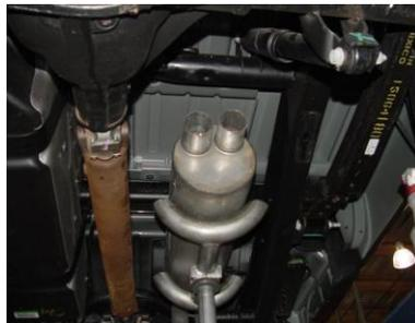
NEXT, INSTALL REAR MUFFLER HANGER #H ONTO DRIVER SIDE OUTLET OF THE MUFFLER. INSERT HANGER INTO RUBBER GROMMET DO NOT TIGHTEN.
