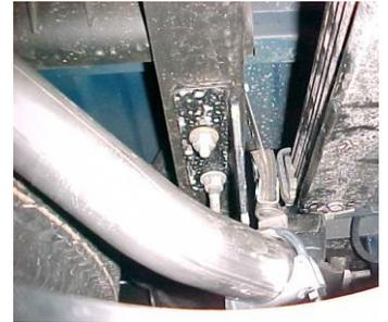
INSTALL PASSENGER SIDE OVER AXLE TAILPIPE #E INTO MUFFLER 1 1/2" TO 2" INSERT WELDED HANGER INTO RUBBER GROMMET. USE CLAMP # J TO SECURE PIPE TO MUFFLER. DO NOT TIGHTEN.
