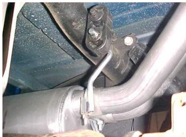
MEASURE 18" FROM THE REAR OF THE FRAME TOWARDS THE FRONT OF THE VEHICLE. USE THIS SLOT FOR THE 10" HANGER #K, INSTALL USING THE 1<sup>ST</sup> HOLE USE HARDWARE KIT PROVIDED.
