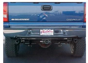
**MAKE SURE YOU HAVE A 1" CLEARANCE FROM ALL BRAKE LINES, SHOCK BOOTS, TIRES, FUEL LINES, ETC...**
