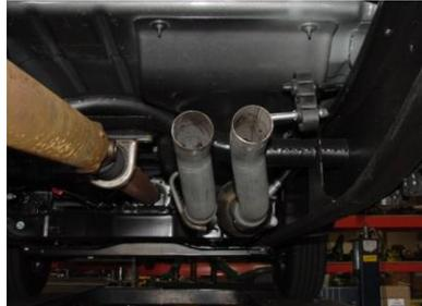
SLIDE MUFFLER #C ONTO HEADPIPES 1-1/2" TO 2" WITH THE INLET FACING THE MOTOR, USE A JACK STAND TO SUPPORT MUFFLER. USE CLAMPS # J TO SECURE MUFFLER TO HEADPIPES. DO NOT TIGHTEN. OUTLETS OF THE MUFFLER SHOULD BE ON THE TOP.
