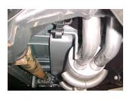
INSTALL EXIT PIPES #F ONTO TAILPIPE. ROTATE EXIT PIPE AND TAILPIPE TO GET THE BEST FIT FOR YOUR VEHICLE WITH PROPER CLEARANCES. USE CLAMP #I TO SECURE TOGETHER. DO NOT TIGHTEN.
