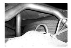
INSTALL PIPE #A ONTO TURBO. SECURE TURBO USING FACTORY CLAMP. INSERT WELDED HANGER INTO RUBBER GROMMET. SNUG TURBO CLAMP BUT **DO NOT TIGHTEN**
