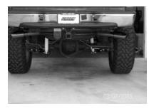
INSTALL YOUR STAINLESS STEEL TIPS TO YOUR DESIRED LOOK AND CLAMP DOWN. WHEN EVERYTHING IS IN PLACE, FIRMLY TIGHTEN DOWN ALL THE BOLTS AND CLAMPS SECURELY STARTING FROM THE FRONT AND WORKING YOUR WAY BACK. TO CLEAN YOUR STAINLESS STEEL TIPS USE A GOOD QUALITY STAINLESS CLEANER.
