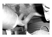
REMOVE THE REMAINING STOCK DOWN PIPE BY UNCLAMPING IT FROM THE TURBO HOUSING. USE A 11MM SOCKET OR WRENCH TO REMOVE YOUR STOCK PIPE THROUGH THE BOTTOM. DO NOT DISGARD THE STOCK CLAMP YOU WILL NEED TO RE-USE IT. NOW, INSTALL YOUR CAT BACK EXHAUST SYSTEM ACCORDING TO THE INSTRUCTIONS PROVIDED IN STEP 2. DO NOT TIGHTEN UNTIL ENTIRE SYSTEM IS INSTALLED.
