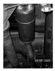
TO INSTALL YOUR **GIBSON DOWN PIPE YOU** NEED TO REMOVE YOUR STOCK EXHAUST FROM THE CAT BACK. REMOVE IT FROM THE 4 BOLT FLANGE IN FRONT OF YOUR STOCK MUFFLER. CUT OFF YOUR STOCK TAILPIPE FOR EASIER REMOVAL. LEAVE ALL RUBBER GROMMETS IN PLACE. USE WD-40 TO AID IN REMOVAL OF EXHAUST AND HANGER MOUNTS.
