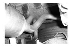
INSTALL DRIVERSIDE OVERAXLEPIPE # E INTO MUFFLER 1 ½"-2". USE CLAMP #L TO SECURE PIPE TO MUFFLER OUTLET. DO NOT TIGHTEN
