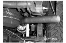
INSTALL PASSENGERSIDE EXIT PIPE #F ONTO TAILPIPE USING CLAMP # L TO SECURE TOGETHER. **DO NOT TIGHTEN.** INSERT WELDED HANGER INTO RUBBER GROMMET, ROTATE IT TO THE BEST FIT FOR YOUR VEHICLE.
