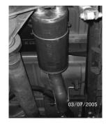
INSTALL MUFFLER #C 1 ½"-2" ONTO PIPE #B. USE CLAMP #K TO SECURE MUFFLER TO PIPE. **DO NOT TIGHTEN**. MAKE SURE MUFFLER OUTLETS ARE LEVEL.
