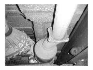
TO INSTALL YOUR GIBSON CAT-BACK YOU NEED TO REMOVE YOUR STOCK EXHAUST FROM THE CAT BACK. REMOVE IT FROM THE 4 BOLT FLANGE IN FRONT OF YOUR STOCK MUFFLER. CUT OFF YOUR STOCK TAILPIPE FOR EASIER REMOVAL. LEAVE ALL RUBBER GROMMETS IN PLACE. USE WD-40 TO AID IN REMOVAL OF EXHAUST AND HANGER MOUNTS.
