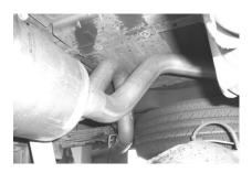
INSTALL DRIVERSIDE OVERAXLEPIPE # D INTO MUFFLER 1 ½"-2". USE CLAMP #K TO SECURE PIPE TO MUFFLER OUTLET. DO NOT TIGHTEN
