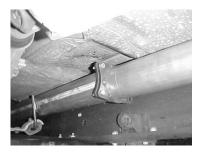
BOLT HEADPIPE #A ONTO FACTORY 4-BOLT FLANGE USING SUPPLIED BOLT KIT #H AND GASKET #I. BEFORE YOU INSTALL MUFFLER INSTALL BAND CLAMP HANGER #L
