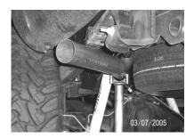
INSTALL DRIVERSIDE EXIT PIPE #F ONTO TAILPIPE. USE CLAMP #K TO SECURE TOGETHER. DO NOT TIGHTEN. INSERT WELDED HANGER INTO RUBBER GROMMET ROTATE TO THE BEST FIT FOR YOUR VEHICLE.
