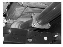
TO INSTALL YOUR GIBSON DOWN PIPE YOU NEED TO REMOVE YOUR STOCK EXHAUST FROM THE CAT BACK. FOR EASIER REMOVAL OF THE **FACTORY MUFFLER CUT** OFF YOUR STOCK TAILPIPE. KNOW REMOVE IT FROM THE 4 BOLT FLANGE IN FRONT OF YOUR STOCK MUFFLER. LEAVE ALL RUBBER GROMMETS IN PLACE. USE WD-40 TO AID IN REMOVAL OF EXHAUST AND HANGER MOUNTS.
