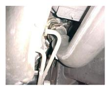
**NSTALL DOWNPIPE #A** ONTO TURBO, SECURE **FURBO USING FACTORY** CLAMP. **NSERT WELDED** HANGER INTO RUBBER **GROMMET. SNUG FURBO CLAMP BUT DO** NOT TIGHTEN ANY OF **THE GIBSON EXHAUST** JNTIL THE VERY END. **SOME MINOR ADJUSTMENTS WILL NEED TO BE MADE FOR A FLAWLESS** INSTALLTION.
