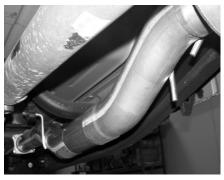
**INSTALL HEADPIPE PIPE# B** ONTO DOWNPIPE ATTACH USING BOLT KIT #I and J. DO **NOT TIGHTEN**
