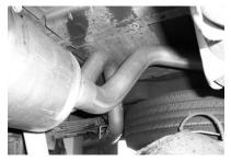
INSTALL DRIVERSIDE TAILPIPE # E INTO MUFFLER 1 1/2"-2". USE CLAMP #L TO SECURE PIPE TO MUFFLER OUTLET.
