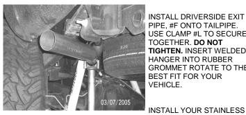
INSTALL DRIVERSIDE EXIT PIPE, #F ONTO TAILPIPE. USE CLAMP #L TO SECURE TOGETHER. DO NOT TIGHTEN. INSERT WELDED HANGER INTO RUBBER GROMMET ROTATE TO THE BEST FIT FOR YOUR VEHICLE.
