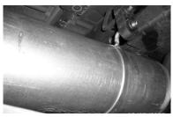
**NEXT ON THE** PASSENGERSIDE & DRIVERSIDE, REMOVE THE HITCH BOLT CLOSEST TO THE FRONT OF THE VEHICLE AND **INSTALL REAR TAILPIPE** HANGERS #N & #O WITH RUBBER GROMMETS #P. LEAVE SNUG UNTIL EXIT PIPES ARE INSTALLED.
