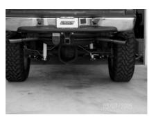
STEEL TIPS TO YOUR DESIRED LOOK AND CLAMP DOWN. WHEN EVERYTHING IS IN PLACE, FIRMLY TIGHTEN DOWN ALL THE **BOLTS AND CLAMPS** SECURELY STARTING FROM THE FRONT AND WORKING YOUR WAY BACK. THE SYSTEM WILL MOVE WHEN BEING TIGHTEND DOWN. WATCH FOR SHOCK CLEARANCE AND FRAME CLEARANCE. TO CLEAN YOUR STAINLESS STEEL TIPS USE A GOOD QUALITY STAINLESS CLEANER.
