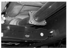
FOR EASIER REMOVAL OF THE STOCK MUFFLER CUT THE FACTORY TAILPIPE JUST BEHIND THE REAR MUFFLER HANGER AND REMOVE. LOCATE THE 4- BOLT FLANGE BEHIND THE FACTORY CONVERTER AND REMOVE THE CAT-BACK. USE WD-40 TO AID IN THE REMOVAL OF **EXHAUST HANGERS**
