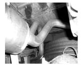
"MAKE SURE YOU HAVE A MINIMUM OF 1" CLEARANCE ON ALL PIPES FROM RUBBER BRAKE LINES, FUEL LINES, TIRES, SHOCKS, ETC..."
