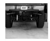
INSTALL DRIVERSIDE EXIT PIPE #G ONTO TAILPIPE. USE CLAMP #L TO SECURE TOGETHER. DO NOT TIGHTEN. INSERT WELDED HANGER INTO RUBBER GROMMET ROTATE TO THE BEST FIT FOR YOUR VEHICLE.
