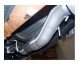
ATTACH HEADPIPE # A ONTO FACTORY EXISTING TURBO DOWNPIPE USING BOLT KIT# I AND GASKET #J. DO NOT TIGHTEN.
