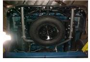
**8.** Install exit pipes #E. Use clamps #G to secure exit pipes to tail pipes. These clamps also attach to the metal hangers. You will need to rotate in order to adjust for clamping.
