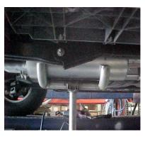
NEXT INSTALL MUFFLER #C. SLIDE IT ONTO HEADPIPE 1-1/2" TO 2". ATTACH TO HEADPIPE WITH CLAMP # G. INLET OF MUFFLER SHOULD FACE TOWARDS THE MOTOR. INSTALL REAR MUFFLER HANGER #J INTO RUBBER GROMMET LOCATED JUST ABOVE THE DRIVERS SIDE OUTLET OF THE MUFFLER. SLIDE CLAMP ONTO MUFFLER OUTLET. INLET OF MUFFLER IS LOOKING INTO THE LOUVERS. DO NOT TIGHTEN.
