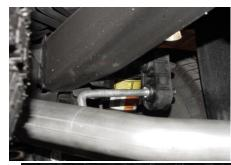
INSTALL PASSENGER SIDE OVERAXLE TAILPIPE # E INTO MUFFLER 1-1/2" TO 2". INSERT WELDED HANGER INTO RUBBER GROMMET. USE CLAMP #I TO SECURE PIPE TO MUFFLER. DO NOT TIGHTEN.
