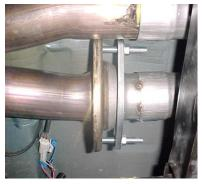
BOLT PASSENGER SIDE HEADPIPE # A USING HARDWARE KIT # L. DO NOT TIGHTEN. INSERT HANGER INTO RUBBER GROMMET, NEXT SLIP DRIVER SIDE HEADPIPE # B ONTO FACTORY PIPE USE CLAMP # G TO SECURE. DO NOT TIGHTEN.
