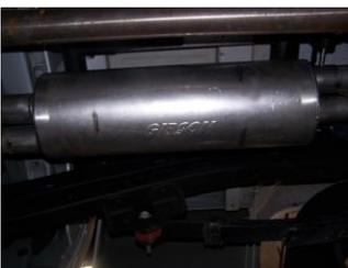
**3.** Install muffler #C onto headpipes 1 1/2"-2" with the louvers facing towards the Y-pipe. Use a jack stand to support the muffler. Use clamp #G to secure the muffler to the headpipes. DO NOT TIGHTEN.
