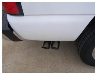
**6.** Install stainless steel tips #F. Clamp down. When you have everything in place, firmly tighten all bolts and clamps down securely. Use stainless steel cleaner and a Scotch Brite pad weekly to prevent tip from discoloration.
