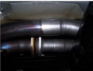
**2.** Install passenger head pipe #A onto stock Y-pipe with bolt kit #I. Use a jack stand to support the headpipe. DO NOT TIGHTEN. Insert welded hanger into rubber grommet. Next install driver headpipe #B onto the factory pipe, secure with clamp #G. DO NOT TIGHTEN.
