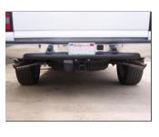
**8.** Install stainless steel tips #H. Clamp down. When you have everything in place, firmly tighten all bolts and clamps down securely. Use zip ties to secure brake/fuel lines away from exhaust. Use stainless steel cleaner and a Scotch Brite pad weekly to prevent tip from discoloration.
