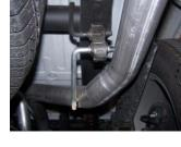
onto muffler 11/2"-2" secure using Insert welded hanger into rubber
