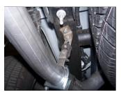
**5.** Attach rear hanger #J to the bottom of the frame about 16" from rear of frame.
