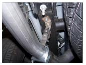
**5.** Attach rear hanger #I to the bottom of the frame about 16" from rear of frame.
