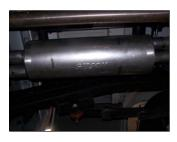
**3.** Install muffler #C onto headpipes 1½"-2" with the louvers facing towards the Y-pipe. Use a jack stand to support the muffler. Use clamp #H to secure the muffler to the headpipes. DO NOT TIGHTEN.
