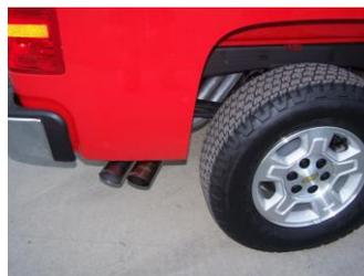
8. Install stainless steel tip. Clamp down. When you have everything in place, firmly tighten all bolts and clamps down securely. Use stainless steel cleaner and a Scotch Brite pad weekly to prevent discoloration. Inspect all fasteners after 25-50 miles of operation and re-tighten as necessary.
