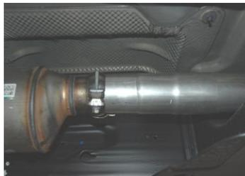
3. Next, install headpipe #A onto your factory flange. Insert welded hanger into the rubber grommet.
