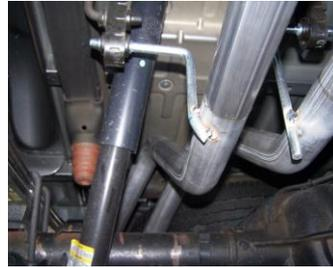
5. Make sure muffler outlets are level before installing tailpipes. Now install passenger tailpipe #C. Insert welded hangers into rubber grommets.
