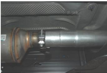
3. Next install headpipe #A onto your factory Flange re-use your factory Nuts insert welded hanger Into rubber grommet
