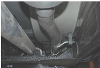
4. Install muffler #B onto head pipe. Use jack stands to support the muffler. Use clamp #F to secure the muffler to headpipe. Do not tighten.
