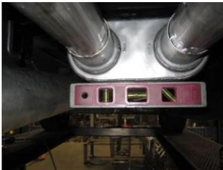
4. Install muffler #B with inlet stands to support the muffler. Use clamp #F to secure the muffler to headpipe. Do not tighten.
