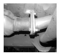
UNBOLT THE FACTORY EXHAUST AT THE FLANGE BEHIND THE CATALYTIC CONVERTER.
