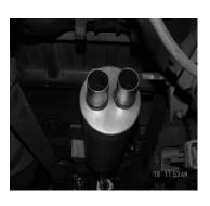
INSTALL MUFFLER #B ONTO HEADPIPE 1-1/2" TO 2". USE CLAMP #G TO SECURE HEADPIPE TO MUFFLER. DO NOT TIGHTEN. USE A JACKSTAND TO SUPPORT MUFFLER.
