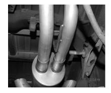
INSTALL TAILPIPES #C & #D INTO MUFFLER 1-1/2" TO 2". INSERT WELDED HANGERS INTO THE RUBBER GROMMETS. USE CLAMP #F AND ATTACH TAILPIPES TO MUFFLER. DO NOT TIGHTEN.
