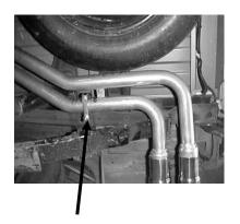
REMOVE FACTORY REAR HANGER FROM THE FRAME ON PASSENGER SIDE. MEASURE ABOUT 19" FROM BACK OF FRAME AND INSTALL #E HANGER USING THE LARGER HOLE. ATTACH WITH CLAMP #F. USE BOLT KIT #H TO CONNECT AND LINE UP TAILPIPES AT REAR TAB.
