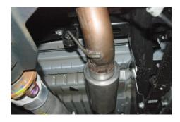
5. Install the over axle pipe Item # C into the muffler outlet. Install hangers into the rubber grommets. You may need to adjust the pipes to allow for proper fitment and clearance. Sometimes these adjustments will be needed at the front head pipes.
