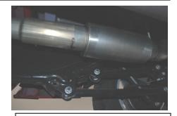
4. Use Clamp Item # E to secure the connection. Do not tighten keep loose for kit adjustment and alignment.
