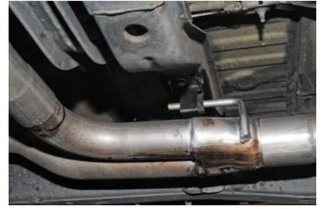
2. Install Head pipe Item # A onto the factory flange. Install hanger into rubber grommet and loosely tighten down the flange.
