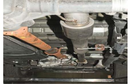
2. Install muffler assembly Item # A into the factory head pipe. You will re use the factory clamp at this connection. Install hanger into rubber grommet and loosely tighten down the clamp.
