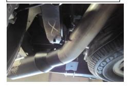
5. With everything loose you may need to adjust the system for proper clearance of shocks, brake lines, ect.
