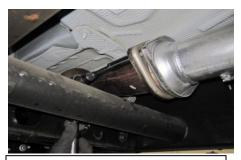
2. Install Head pipe# A onto the factory flange. You will re use the factory nuts at this connection. Loosely tighten down the flange.
