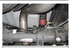
4. Install over axle pipe Item # C into the muffler outlet. Slip the hangers into the rubber grommets and keep tailpipe loose. Use clamp #F to secure tailpipe to the muffler.
