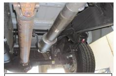
3. Install muffler assembly Item # B onto the head pipe. You may need to use a jack stand to support the muffler while installing the tailpipe. Use Item# E to clamp the muffler assembly to the head pipe. Loosely tighten down. Insert hanger into rubber grommets.
