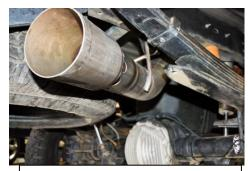
6. Install The Exhaust tip. The kit was designed to have a 1" clearance from the bottom of the quarter panel.
