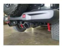
7. Adjust the tips to your preference. Make sure everything is clear of frame rails and parts and re tighten the system starting from the front clamp. Check everything after each clamp is tightened.
