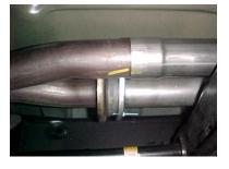
Install passenger side headpipe # A onto stock flange using hardware provided, do not tighten. Insert welded hanger into rubber grommet. Next, install driver side headpipe # B onto stock pipe, use clamp # G to secure together, do not tighten.
