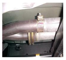
Lay out the exhaust on the floor so it looks like the drawing and compare parts with manual. To remove the stock exhaust remove it from the stock flange & slip joint located in front of the muffler, then cut off your tailpipe just behind the muffler. Use WD-40 to aid in removal of hangers from grommets leave grommets on vehicle.
