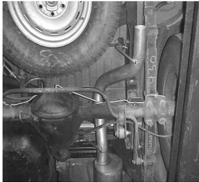
INSTALL THE OVERAXLE TAILPIPE #C INTO MUFFLER AT LEAST 1 1/2" TO 2" USING CLAMP #F . DO NOT TIGHTEN. INSERT WELDED HANGERS INTO RUBBER GROMMETS. THE SPARE TIRE ON SOME VEHICLES MAY NEED TO BE LOOSENED AND PULLED TO THE DRIVER SIDE AND RE-TIGHTENED. ROTATE PIPES UNTIL YOU HAVE AT LEAST A 1" CLEARANCE AWAY FROM ALL PIPES, ETC.
