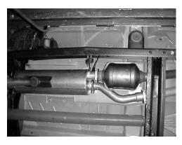
AFTER STOCK EXHAUST IS REMOVED, INSTALL DRIVERSIDE HEADPIPE #A ONTO STOCK HEADPIPE USING CLAMP #H. INSERT HANGER INTO THE RUBBER GROMMET ON THE PASSENGERSIDE CONNECT DUAL INLET MUFFLER WITH CLAMP #H ON THE PASSENGERSIDE AND CLAMP #F ON THE DRIVERSIDE WITH HEADPIPES AND ONTO THE BACK OF THE STOCK CONVERTER. DO NO TIGHTEN KEEP MUFFLER AWAY FROM THE FRAME. OUTLET OF MUFFLER WILL BE AT ABOUT 7-8 O'CLOCK POSITION.
