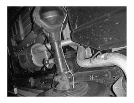
LAY THE GIBSON EXHAUST SYSTEM LIKE IT IS SHOWN ON INSTRUCTION MANUAL AND MAKE SURE ALL PIPE NUMBERS MATCH THE INSTRUCTION NUMBERS. REMOVE O2 SENSER CUTTING BEFORE STOCK HEADPIPE OR TAILPIPE. FOR EASIER REMOVAL OF 02 SENSER. LUBRICATE WITH WD-40 ON PASSENGER SIDE. CUT STOCK TAILPIPE ON THE PASSENGER SIDE JUST BEHIND THE STOCK
