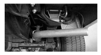
SLIP TURNOUT PIPE #D ON TO TAILPIPE USING CLAMP #G. NOW ROTATE TURNOUT PIPE AND INSTALL STAINLESS STEEL TIP TO DESIRED LOOK.. USE AN ALUMINUM OR STAINLESS STEEL CLEANER TO POLISH TIP. MAKE SURE YOU HAVE 1" CLEARANCE ON ALL PIPES FROM ALL RUBBER BRAKE LINES, SHOCK BOOTS, TIRES, ETC.. TIGHTEN ALL CLAMPS DOWN. THEN REINSTALL THE O2 SENSER. BE CAREFUL NOT TO CROSS THREAD OR DAMAGE THE SENSOR.
