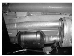
BRACE STOCK CATALYTIC CONVERTER SO IT DOES NOT REST ON CROSSMEMBER. THEN ON PASSANGER SIDE CUT 2 1/2" BEHIND THE WELD ON THE CONVERTER. THEN ON THE DRIVER SIDE CUT 17 ½ BEHIND FLANGE. NOW YOU CAN REMOVE STOCK MUFFLER, HEADPIPES, AND TAILPIPES.
