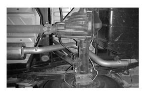
NOW INSERT OVERAXLE TAILPIPE #C AND INSERT INTO WELDED HANGER STOCK RUBBER GROMMETS BEHINDTHE MUFFLER.STAIGHTEN TAILPIPE OUT AND INSERT INTO REAR OF THE MUFFLER NO LESS THAN 1-1/2" AND NO MORE THAN 2" USING CLAMP #G. DO NOT TIGHTEN
