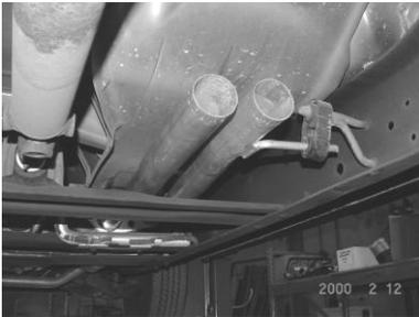
BOLT HEADPIPE #A USING SUPPLIED FLANGE GASKET #H AND REUSING FACTORY BOLTS. APPLY A SMALL AMOUNT OF HIGH-TEMP O2 SENSOR SAFE SILICONE ON THE FLANGE TO PREVENT ANY LEAKS. INSERT WELDED HANGER INTO RUBBER GROMMET. DO NOT TIGHTEN
