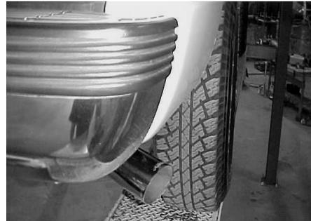
INSTALL TURNOUT PIPE #D INTO TAILPIPE USING CLAMP #G . INSTALL THE STAINLESS TIP AND CLAMP DOWN. USE ANY STAINLESS STEEL OR ALUMINUM CLEANER TO POLISH TIP.
