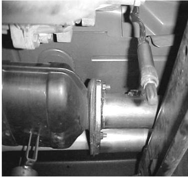
REMOVE O2 SENSOR FROM STOCK HEAD PIPE AND UNBOLT STOCK HEAD-PIPE. YOU WILL REUSE YOUR STOCK NUTS AND BOLTS. CUT STOCK EXHAUST JUST BEHIND THE MUFFLER FOR EASIER REMOVAL. LEAVE ALL RUBBER GROMMETS IN PLACE. FOR EASIER REMOVAL OF HANGERS SPRAY WD-40 TO AID YOU IN REMOVING THEM.
