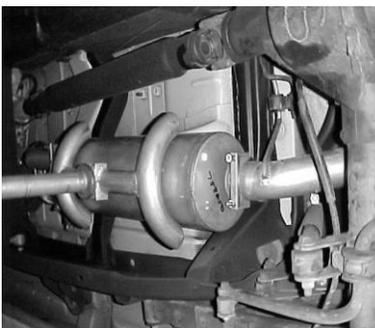
SLIDE MUFFLER WITH DUAL INLET ONTO HEADPIPE AT LEAST 1-1/2" TO 2". MUFFLER OUTLET SHOULD BE AT THE 5 O'CLOCK POSITION. USE CLAMPS #F TO ATTACH TO THE HEADPIPE. MAKE SURE INLETS AND THE MUFFLER IS LEVEL. AND TIGHTEN DOWN. USE JACK STAND TO SUPPORT MUFFLER.
