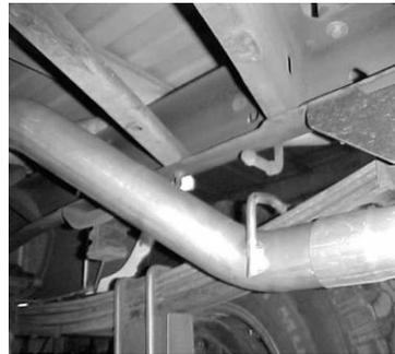
INSTALL THE OVERAXLE TAILPIPE #C INTO MUFFLER AT LEAST 1 1/2" TO 2" USING CLAMP #G . DO NOT TIGHTEN. INSERT WELDED HANGERS INTO RUBBER GROMMETS. THE SPARE TIRE ON SOME VEHICLES MAY NEED TO BE LOOSEN ED AND PULLED TO THE DRIVER SIDE AND RE-TIGHTENED. ROTATE PIPES UNTIL YOU HAVE AT LEAST A 1" CLEARANCE AWAY FROM SHOCK, BRAKE LINES, SPARE TIRE, ECT.
