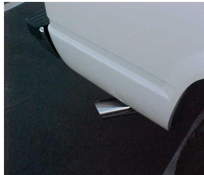
INSTALL TURNOUT PIPE #D INTO TAILPIPE USING CLAMP #G . INSTALL THE STAINLESS TIP AND CLAMP DOWN. USE ANY STAINLESS STEEL OR ALUMINUM CLEANER TO POLISH TIP. TIGHTEN ALL NUTS ,BOLTS AND CLAMPS.
