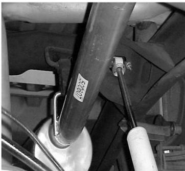
SLIDE MUFFLER WITH DUAL INLET ONTO HEADPIPE AT LEAST 1-1/2" TO 2". MUFFLER OUTLET SHOULD BE AT THE 12 O'CLOCK POSITION. USE CLAMPS #F TO ATTACH TO THE HEADPIPE. MAKE SURE INLETS AND MUFFLER IS LEVEL. AND TIGHTEN DOWN. USE JACK STAND TO SUPPORT MUFFLER.
