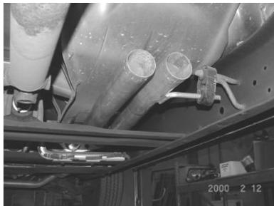
BOLT HEADPIPE #A USING SUPPLIED FLANGE GASKET #G AND REUSING FACTORY BOLTS. APPLY A SMALL AMOUNT OF HIGH-TEMP O2 SENSOR SAFE SILICONE ON THE FLANGE TO PREVENT ANY LEAKS. INSERT WELDED HANGER INTO RUBBER GROMMET. DO NOT TIGHTEN
