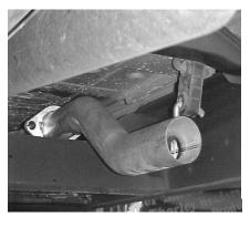
BOLT HEADPIPE #A TO THE STOCK FLANGE RE-USING THE FACTORY NUTS & BOLTS AND FLANGE GASKET# G. INSERT WELDED HANGER INTO RUBBER GROMMET.
