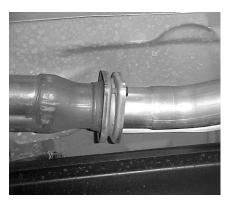
UNBOLT THE STOCK EXHAUST AT THE FLANGE BEHIND THE Y-PIPE AND REMOVE. MAKE SURE TO LEAVE ALL RUBBER GROMMETS IN THE FACTORY LOCATION. YOU WILL RE-USE STOCK NUTS AND BOLTS. FOR EASIER REMOVAL OF EXHAUST, CUT BEHIND THE MUFFLER. USE WD-40 TO REMOVE HANGERS FROM GROMMETS.
