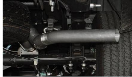
INSTALL EXIT PIPE #E ONTO TAILPIPE. INSERT WELDED HANGER INTO RUBBER GROMMET. USE CLAMP #H TO SECURE THE EXIT PIPE TO THE TAILPIPE. DO NOT TIGHTEN. ROTATE THE PIPE UNTIL IT IS LEVEL.
