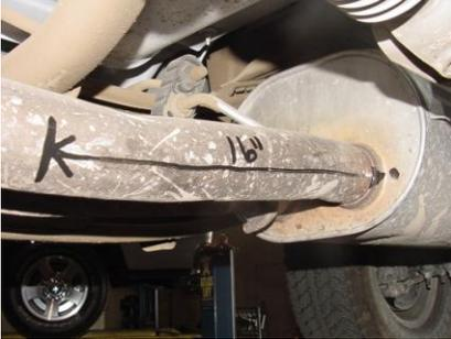
TO REMOVE YOUR STOCK EXHAUST, MEASURE 16" FROM THE MUFFLER FORWARD TOWARDS THE FRONT OF THE VEHICLE. LEAVE ALL RUBBER GROMMETS ON THE HANGER. USE WD-40 TO AID IN THE REMOVAL OF THE EXHAUST AND HANGERS
