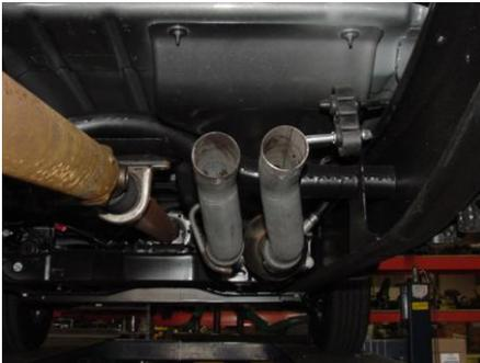
SLIDE HEADPIPE #A ONTO STOCK PIPE. INSERT WELDED HANGER INTO RUBBER GROMMET. SLIDE HEADPIPE #B ONTO STOCK PIPE USING CLAMP #I TO SECURE BOTH HEADPIPES. DO NOT TIGHTEN.
