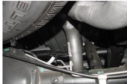
AFTER YOU HAVE CHECKED FOR PROPER CLEARANCES YOU CAN TIGHTEN ALL CLAMPS STARTING FROM THE FRONT AND WORKING YOUR WAY BACK.
