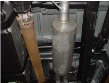
INSTALL MUFFLER #C ONTO HEADPIPE AT LEAST 1-1/2" TO 2". MUFFLER OUTLET WILL BE AT THE 12 O'CLOCK POSITION. USE CLAMP #G TO SECURE THE MUFFLER TO BOTH HEADPIPES. DO NOT TIGHTEN.
