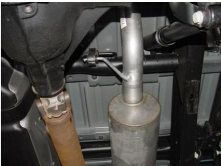
INSTALL TAILPIPE #D INTO MUFFLER 1-1/2" TO 2". INSERT WELDED HANGER INTO RUBBER GROMMET. USE CLAMP #H TO SECURE TAILPIPE #D TO MUFFLER. DO NOT TIGHTEN.
