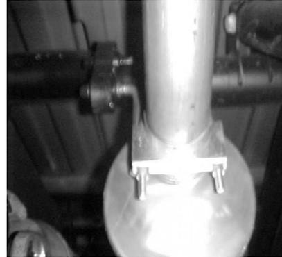
INSTALL REAR MUFFLER HANGER # F ONTO OUTLET OF MUFFLER. INSERT HANGER INTO RUBBER GROMMET.
