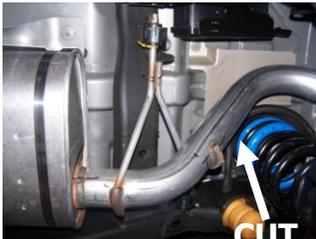
**2.** To remove the stock exhaust, remove it from the two bolt flange in front of the muffler. Do not discard you will re-use bolts. Disengage the welded hangers using WD-40 from the OEM rubber grommets. Do not damage or remove the rubber grommets as you will reuse them to mount your new system. Now, cut off tailpipe before and after rear axle for removal.
