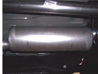
**4.** Install muffler #B onto head pipe #A 1 1/2"-2". Use a jack stand to support the muffler. Use clamp #E to secure the muffler to the headpipe. Do not tighten. Muffler outlet will be in the 11 o'clock position.
