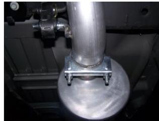
**7.** Install stainless steel tip. Clamp down.
