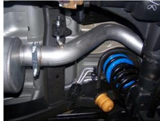
**5.** Install overaxle tailpipe #C into muffler. Insert welded hangers into rubber grommets.
