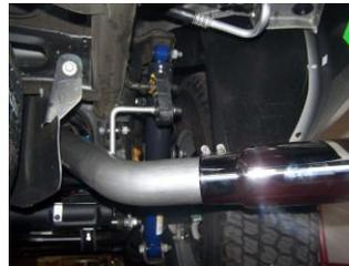
**6.** Use clamp #E to secure tailpipe to the muffler. DO NOT TIGHTEN.
