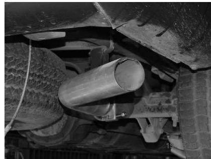
INSTALL OVERAXLE TAILPIPE #C INTO MUFFLER 1-1/2" TO 2" USING CLAMP #F TO SECURE THE TAILPIPE TO THE MUFFLER.
