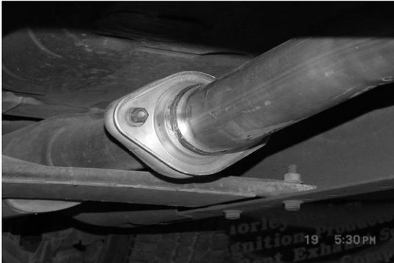
UNBOLT THE 2 BOLT FLANGE LOCATED BEHIND THE CATALYTIC CONVERTER. **SAVE STOCK NUTS AND BOLTS. YOU WILL REUSE THEM.**
