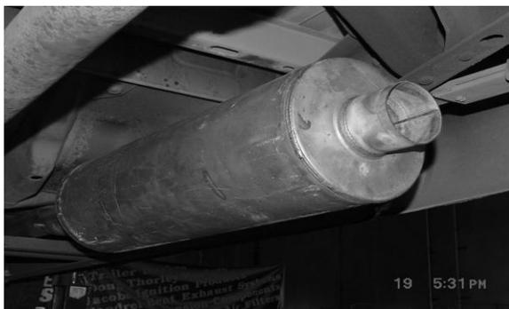
SLIDE MUFFLER ONTO HEADPIPE 1-1/2" TO 2" USING CLAMP #F TO SECURE MUFFLER TO HEADPIPE. USE A JACKSTAND TO SUPPORT MUFFLER. DO NOT TIGHTEN. MUFFLER INLET IS LOOKING INTO THE LOUVERS.
