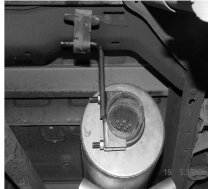
INSTALL REAR MUFFLER O.E. HANGER #H INTO RUBBER GROMMET AND SLIDE IT ONTO THE MUFFLER OUTLET. DO NOT TIGHTEN.
