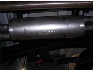
**3.** Install muffler #C onto headpipes 1 1/2"-2" with the louvers facing towards the Y-pipe. Use a jack stand to support the muffler. Use clamp #G to secure the muffler to the headpipes. DO NOT TIGHTEN.
