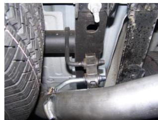
**5.** Next, insert the welded hanger from over axle pipe into rubber grommet. Rotate pipe for proper angle and clearance.
