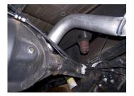
muffler. Use clamp #E to secure the muffler to the headpipe. Do not tighten. Muffler inlet is looking into the louvers.
