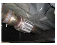
2. Remove the stock exhaust by unbolting it at the clamp Disengage the welded hangers from the OEM rubber grommets. Use WD-40 to aid in this process. Do not damage stock nuts and bolts or remove the rubber grommets as you will re-use them to mount your new system. Now, cut off tailpipe and remove system.
