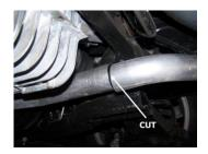
2. To remove stock exhaust, cut it on each side just after the bend before it goes under the rear end. Do not damage or remove the rubber grommets as you well re-use them to mount your new system.
