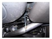
3. Install passenger side muffler assembly #B. Insert welded hangers into rubber grommets. Use clamp #C to secure pipes together. Do not tighten.
