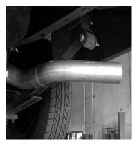
INSTALL EXIT PIPE #C ONTO THE OVER AXLE PIPE USING CLAMP #E. DO NOT TIGHTEN. NOW ROTATE PIPE'S UNTIL YOU HAVE A MINIMUM OF A 1" CLEARANCE ON ALL PIPE'S FROM ALL BRAKE LINES, TIRES, FUEL LINES, SHOCK BOOTS, ETC. THEN TIGHTEN ALL CLAMPS AND HANGERS.
