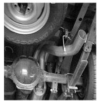
INSTALL OVER AXLE PIPE #B INTO THE OUTLET OF THE MUFFLER 1-1/2" TO 2". INSERT REAR WELDED HANGER INTO THE FACTORY RUBBER GROMMET USING HANGER #G. IF NEEDED ALSO USE CLAMP #E AT THE OUTLET OF THE MUFFLER. DO NOT TIGHTEN.
