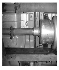
IN FRONT OF THE STOCK HEADPIPE INSTALL BAND CLAMP PART #H INTO RUBBER GROMMETS.SLIP MUFFLER #A ONTO THE FACTORY HEADPIPE NO MORE THEN 2" AND NO LESS THEN 1 ½". INLET HAS LOUVERS FACING THE MOTOR. USE CLAMP # F AT THE INLET OF THE MUFFLER. ATTACH IT TO THE FACTORY HEADPIPE. DO NOT TIGHTEN. USE A JACK STAND TO SUPPORT THE MUFFLER.
