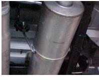
SLIDE BAND CLAMP #G ONTO MUFFLER #B. INSERT HANGERS INTO RUBBER GROMMETS. SUGGESTED TOOLS:
